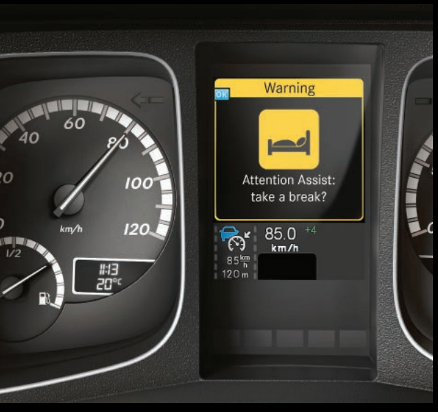
Attention Assist. Monitors the attention paid by the driver. It is based on the Lane Keeping Assist system. The attention paid by the driver is measured on the basis of the driver staying in-lane, in combination with various driver activities (direction indicator/accelerator/engine brake/retarder operation, etc.) as well as steering behaviour.
