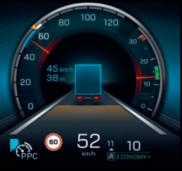
Proximity Control Assist 1) . The safety system with stop-and-go function is on hand to support the driver in stressful situations and can reduce the risk of rear- end collisions.
